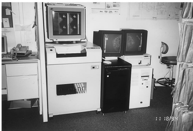
Fig. 24. An intelligent CAD workstation for computerized detection of masses and clustered microcalcifications, which includes a laser film digitizer, a high-speed computer, high-resolution monitors, and a video printer.
